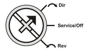
Fig. 3. Rotation Direction Switch
