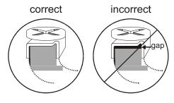
Fig. 6. Correct/incorrect tightening of end limits
