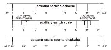
Fig. 7. Internal auxiliary switch triggering points
