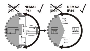
Fig. 8. Mounting for IP54/NEMA2
